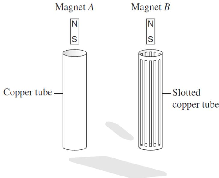
The magnets are dropped simultaneously. Each magnet falls straight through its tube without touching the tube walls.
